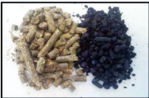
Figure 8 display pellets and bio char made from dried WSG.
