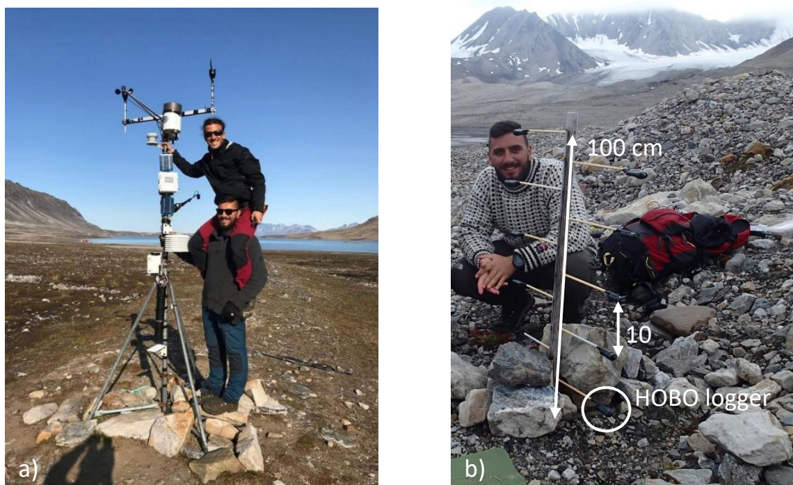
Figure 2 a) The main weather station in Linné valley from where temperature and radiation were collected for the study b) The snow tree located near Linné glacier that is recording snow height and temperature. Photos: AL Werner
