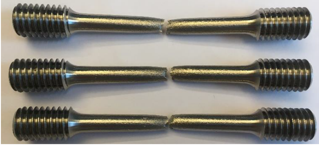
Figure 3.2: Tensile tested specimens produced using SLM additive manufacturing method.
