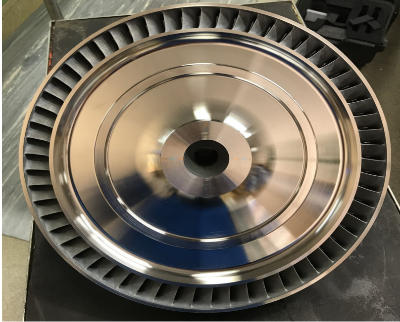
Figure 1.1: Prometheus demonstrator rotor.
