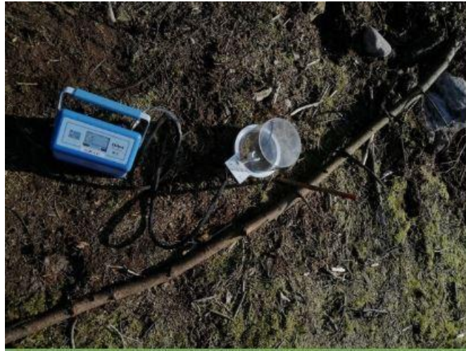
Figure 4.3: EGM-5 portable gas analyzer with transparent CPY-5 chamber used for closed measurement. The chamber was measuring PAR as well.
