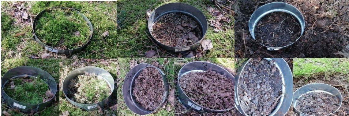
Figure A1: surface covers (vegetation cover, bare soil layer and mineral layer) and the three replicates for the forest plots with the aluminum rings inserted. a) from the left displays the vegetation surface cover, b) is the bare soil layer and c) is the mineral layer
