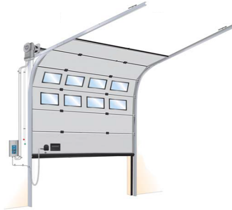
Figure 2.7: Figure shows a general sketch of an Overhead Sectional Door [8].
