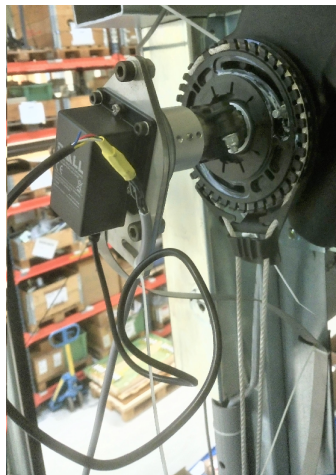
Figure 2.6: Figure shows the mounting of the encoder.
