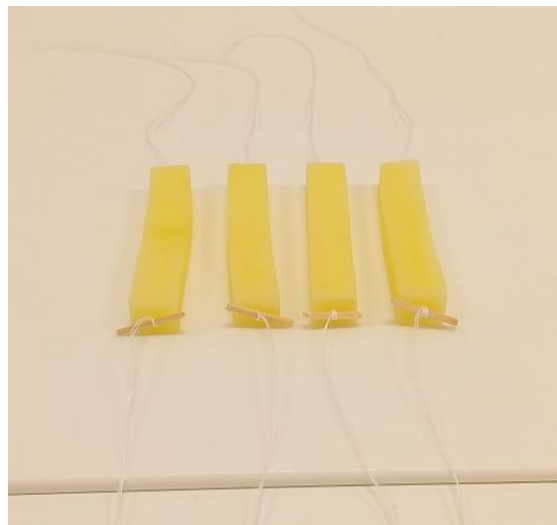
Figure 4. slices of potato with a thread sewn into each piece and fastened at the bottom using a toothpick.
