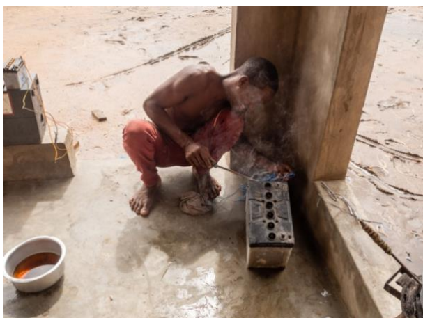
Picture 16, 17, 18 & 19: Joseph making positive poles for battery; untangling a ripped plastic bag; closing up the battery by melting the plastic; tools heating up in cooking stove. Madzedze. Zoe Elsner.
