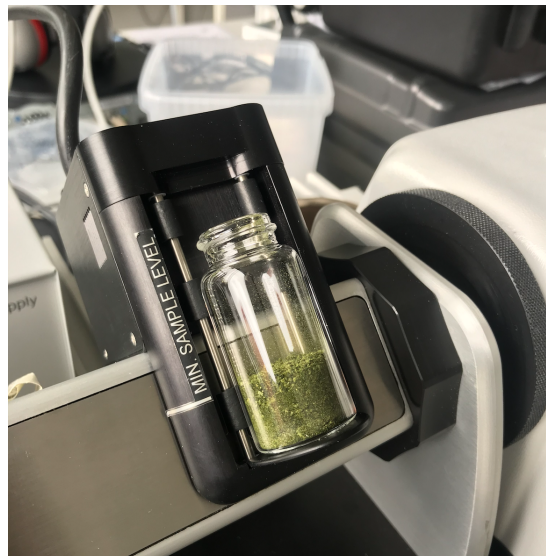
Figure 17 Rotating glass vial on FT-NIR. The glass vial is filled up at least to the minimum required sample level to cover the entire light beam. Photo: Christina A Andersen, 2020
