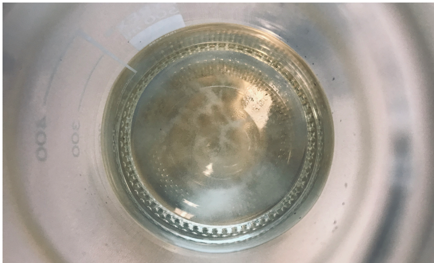
Figure 16 Ethanol precipitated soluble material before filtration within the enzyme assay. Photo: Christina A Andersen, 2020.
