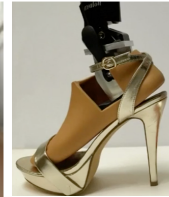
STUDENTS FROM JOHNS HOPKINS UNIVERSITY - Adjustable Prosthetic Foot for High Heels Unfortunately, there is not a lot of information about this one out there but it seems to work like the one from Freedom Innovation.
