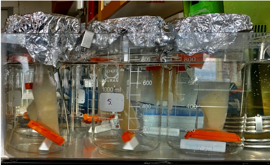
Figure 4: Dialysis tubes incubated in amylase buffer at 37° C on a magnetic stir plate
