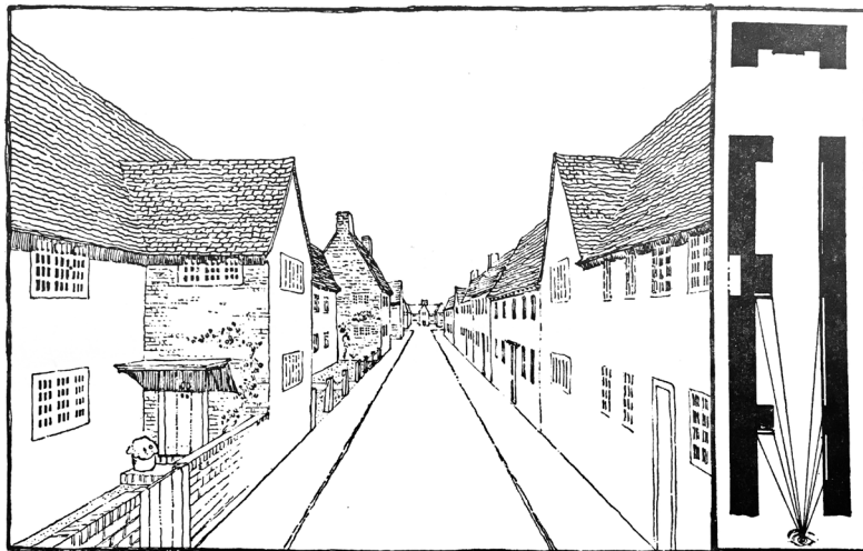
Illus. 191.—Plan and sketch of street showing on one side the uninteresting vanishing perspective of the unbroken building line, and on the other the more picturesque result of breaks.
