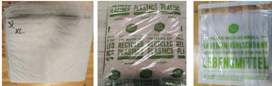
Figure 2-2: Cooling pouches, (a) paper-based (UK), (b) PET and (b) PE (city pouch).
