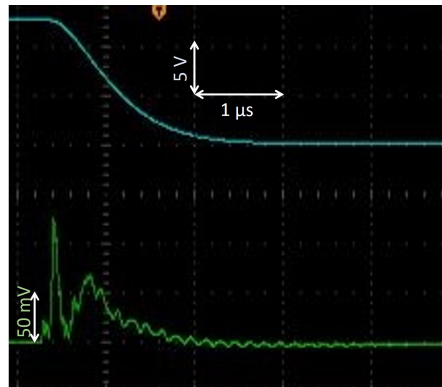
Figure 16: Oscilloscope readout from the 38 mm diameter, primary coil (upper trace) and DSC (lower trace). The initial interference between primary and secondary coil is seen as the large peak at start of DSC trace. The current through the primary coil takes longer time to decay to zero than for smaller the diameter coils, \sim 2.5 \mu\text{s} .
