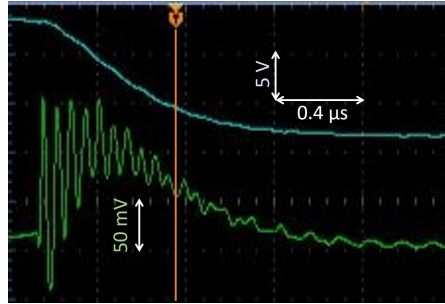
Figure 15: DSC setup, damping resistor in series, with Al rod sample. Data from measurement after rewinding of primary coil. The vertical line is the trigger line. The upper trace is the primary coil circuit voltage and the lower trace is the DSC circuit voltage. The current through the primary coil has a decay time \sim 1.2 \mu\text{s} .
