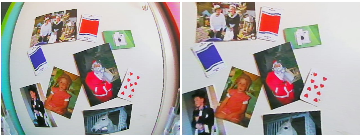
Figure 4.3: An example image from the data set Pictures . The left image is the original and the right is after the image has been undistorted.
