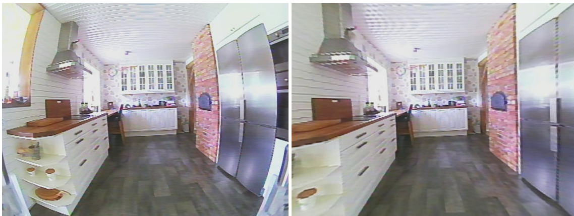
Figure 4.8: An example image of the Kitchen data set. The left image shows the original and the right shows the same image after it has been undistorted.
