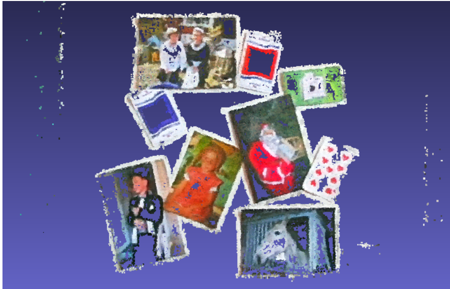
Figure 4.2: Dense reconstruction by COLMAP of the Pictures data set. Visualized in Meshlab.
