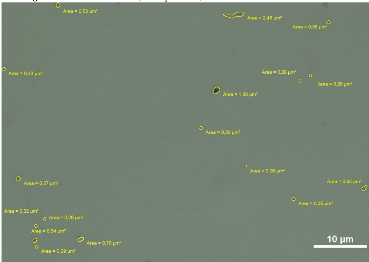
Figure E.15: 347H first area particles, heat treated at 1230°C. Cross-sectional view
