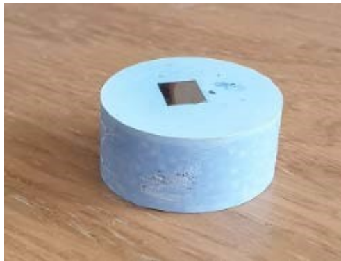
Figure 4.1: An example of a stainless-steel sample molded into an epoxy puck
