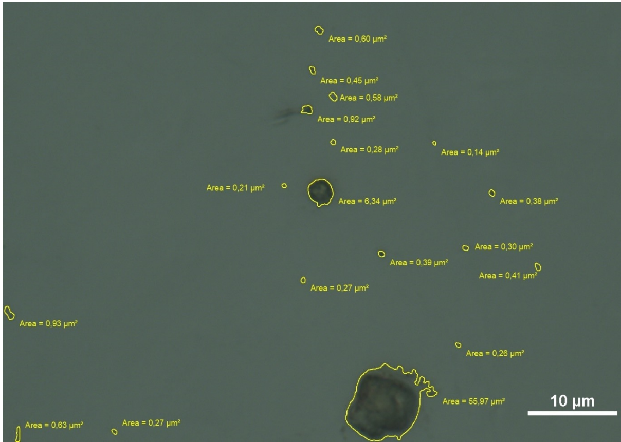
Figure E.16: 347H secondary area particles, heat treated at 1230°C. Cross-sectional view
