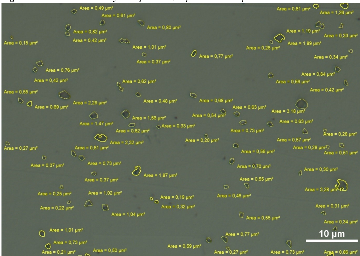
Figure E.13: 347H first area particles, heat treated at 1230°C. Planar view
