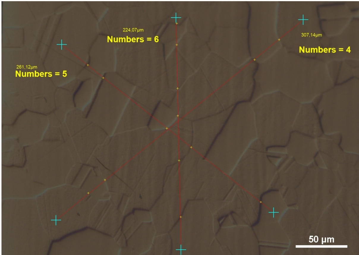
Figure D.5: 316 in the cross-sectional direction, heat treated at 1020°C
