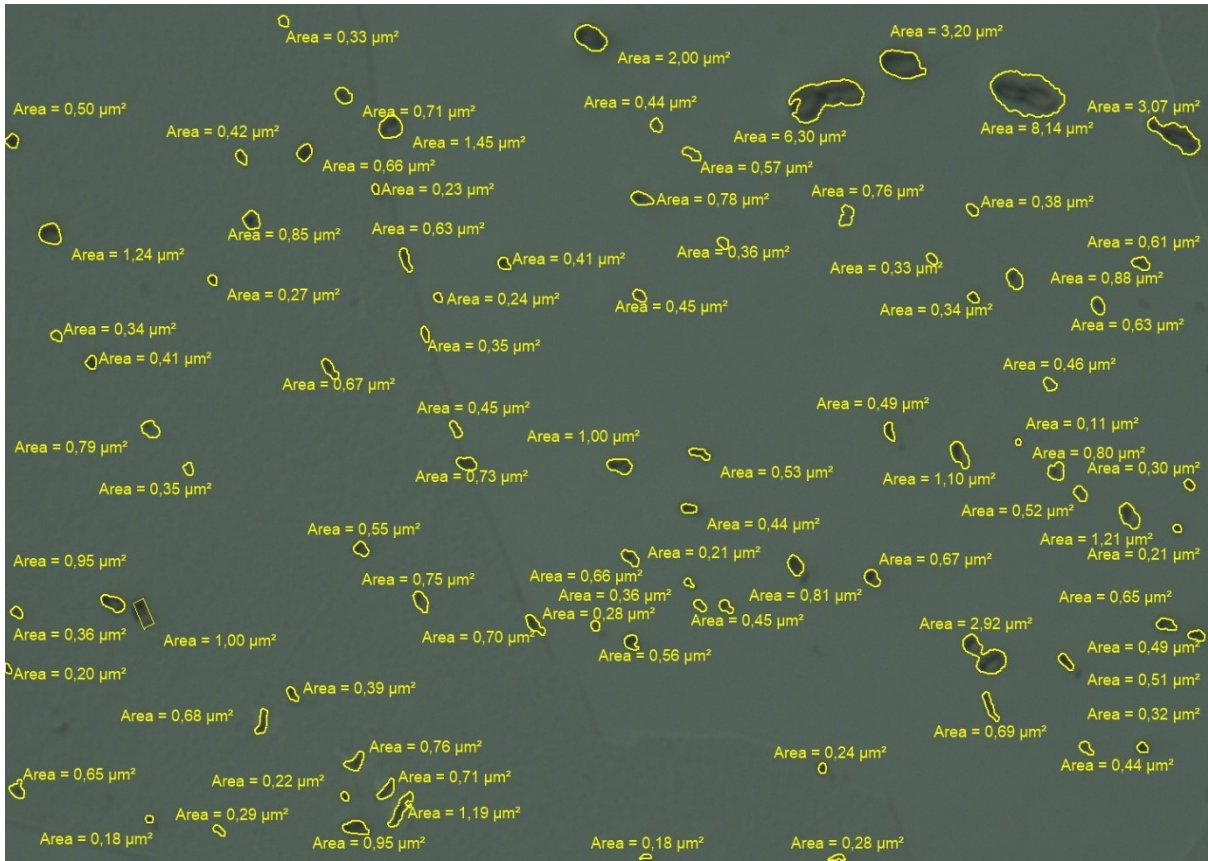
Figure E.14: 347H secondary area particles, heat treated at 1230°C. Planar view
