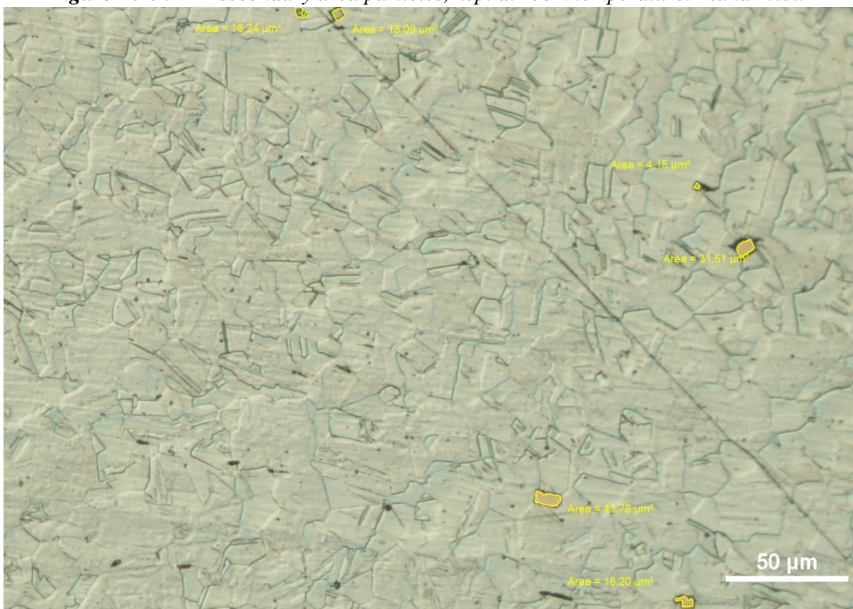
Figure E.3: 321H first area particles, kept at room temperature. Cross-sectional view
