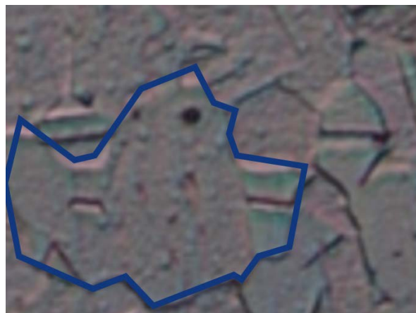
Figure 1.1: An example of a grain in stainless steel
