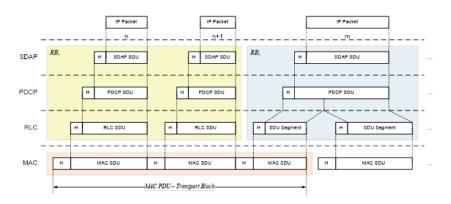
Figure 2.4: Header structure for 5G NR release 15 [8].
