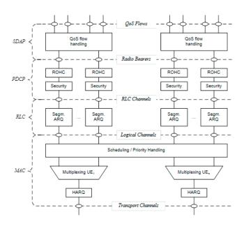
Figure 2.3: Layer-2 protocol stack for 5G uplink [8].
