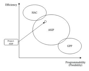
Figure 2.5: ASIP vs GPP and HAC [12].
