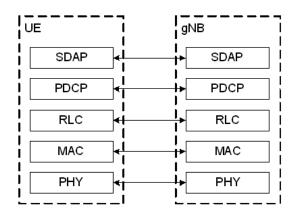
Figure 2.2: User and control-plane protocol stack[8].
