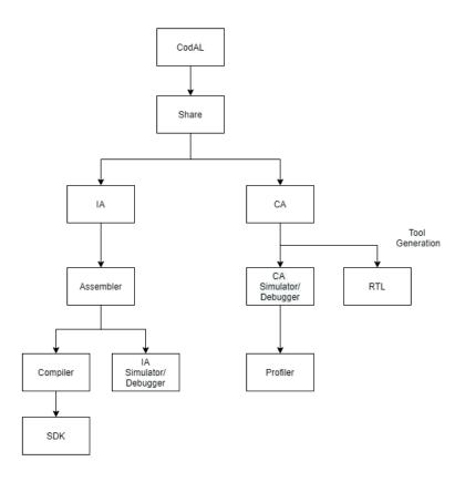
Figure 2.7: Codasip flowchart
