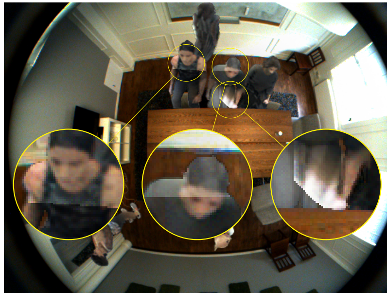
Figure 5.14: Reinsertion artifacts where overlapping image crops have conflicting refinements, resulting in sharp borders.
