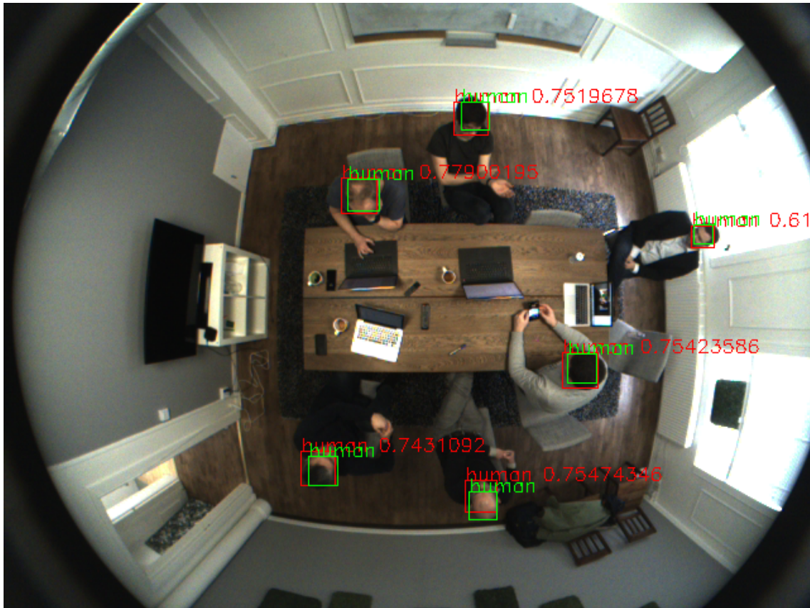
Figure 2.19: SqueezeDet detections. Boxes in green are ground truth labels. Boxes in red are the network’s predictions, along with the respective predicted confidence scores.
