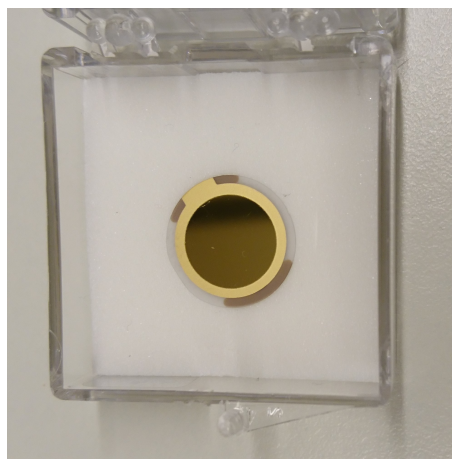
(c) Quartz crystal sensor with gold surface.
