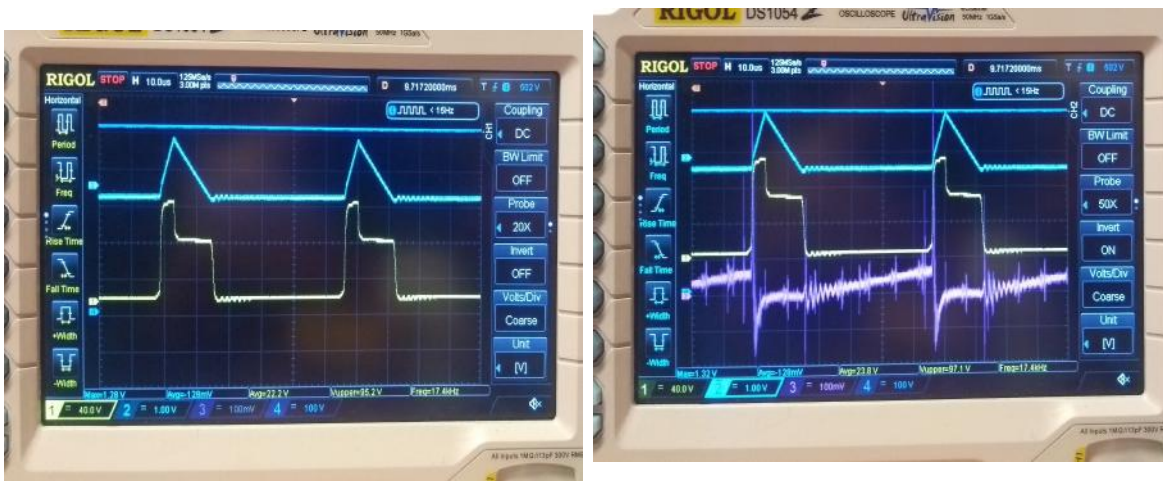
(a) Cyan: secondary current. Yellow: Power transistor collector voltage. Purple: primary current measurement. (b) Cyan: secondary current. Yellow: Power transistor collector voltage. Purple: primary current measurement.
