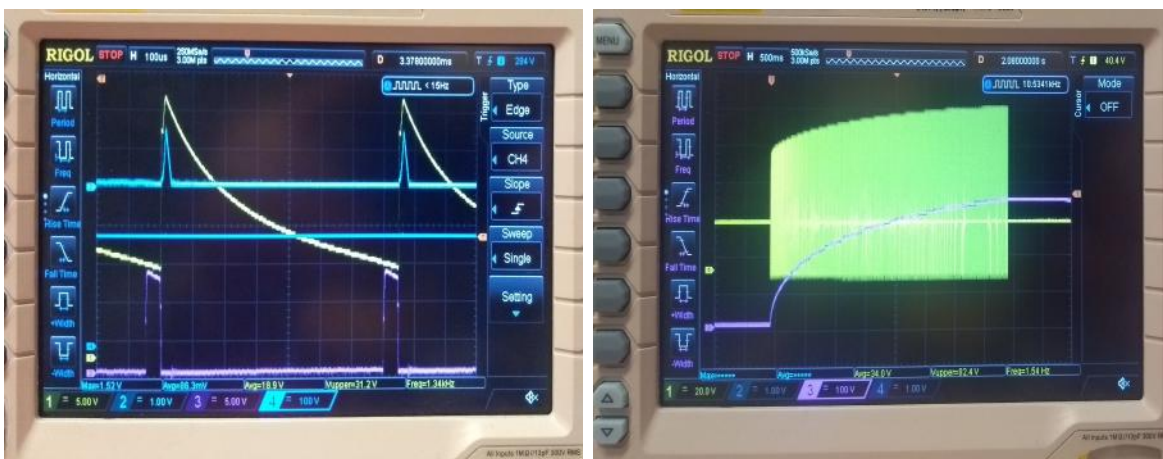
(a) Cyan: secondary current. Yellow: V_{DCM} (b) Cyan: secondary current. Yellow: V_{DCM}
