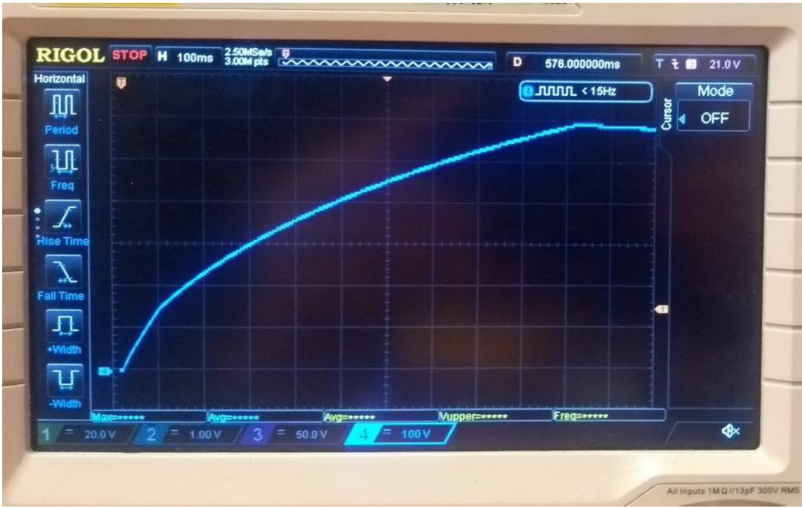
Figure 6.6: Output capacitor voltage when in PCDC
