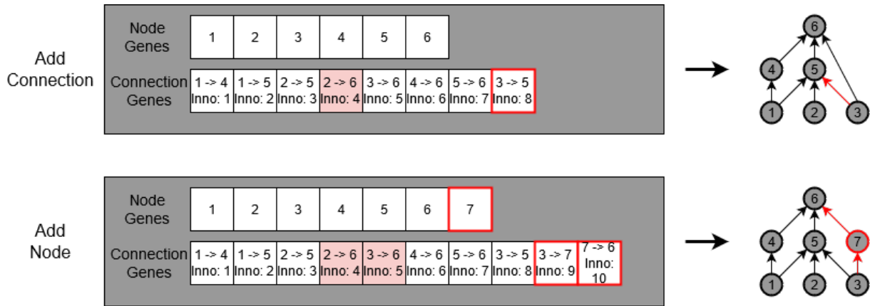
Figure 2.4: Shows a schematic representation of how the genome of an individual is encoded and decoded in NEAT. It also shows how structural mutations affect the genome. Genes with the red border represent a newly added gene, while genes with a red background are disabled genes, i.e. not expressed in the network. Adding a connection adds 1 new connection gene, and adding a new node adds 1 new node gene and 2 new connection genes as well as disabling the connection gene that the node was added on top of.
