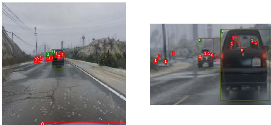
Figure 2.4: Filtered and saved bounding boxes in the GTAV dataset. Red bounding boxes are removed while green are kept. Numbers represents the class indices. For example: 0 is car, 1 is person.
