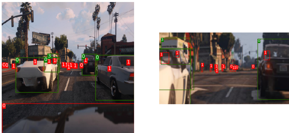
Figure 2.3: Filtered and saved bounding boxes in the GTAV dataset. Red bounding boxes are removed while green are kept. Numbers represents the class indices. For example: 0 is car, 1 is person.
