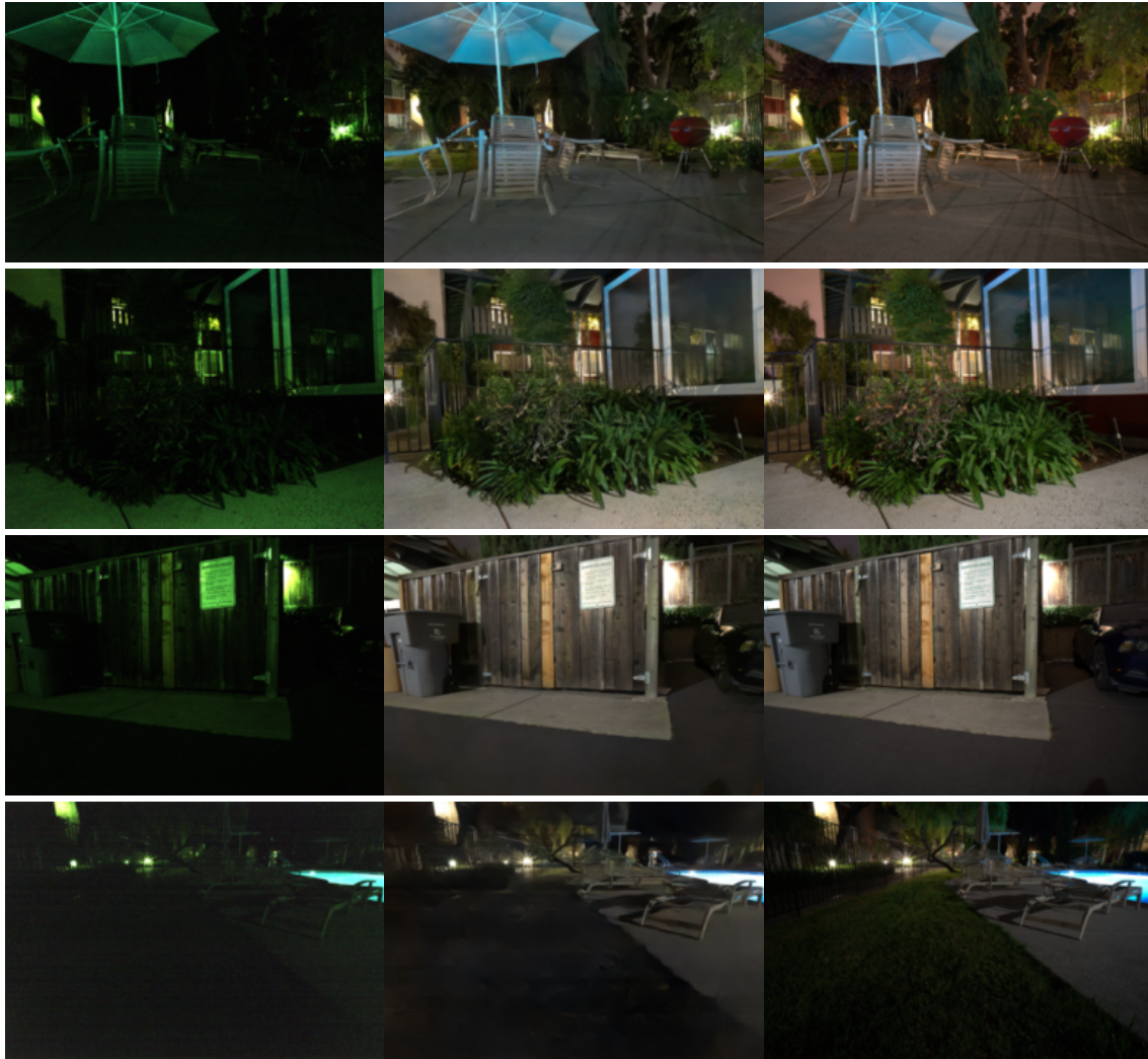
Figure 17: Full-sized predictions of the baseline CVAE SID-net , together with corresponding ground truth. The order is 1) input RAW (amplified), 2) SID-net prediction, 3) ground truth. The first input has ISO 2000, so has the second one. The third one has ISO 320, and the last one 1600.
