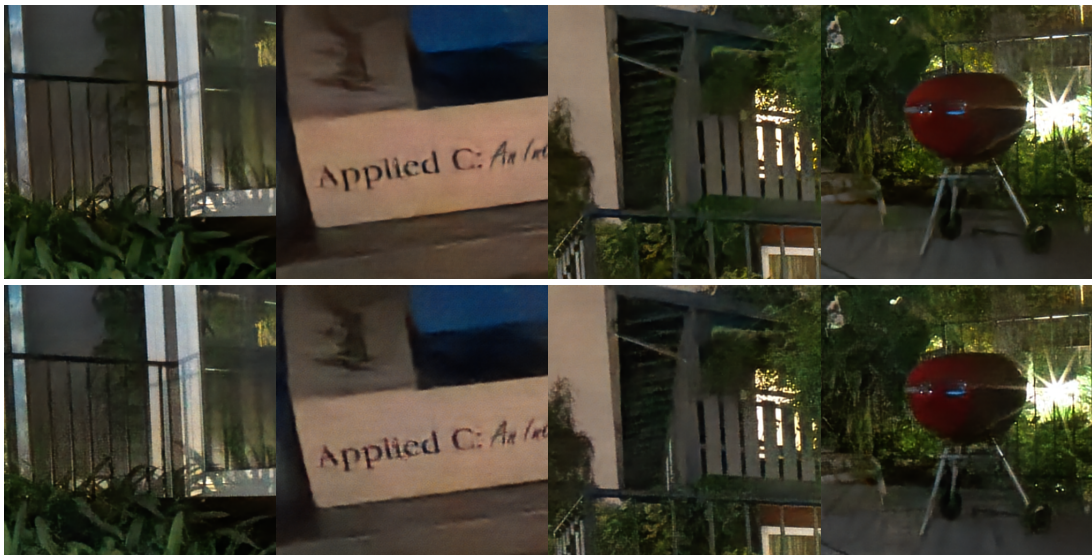
Figure 25: Comparison of the baseline SID-net with SID-net small . Order is: 1) SID-net , 2) SID-net small . These are crops of size 512 \times 512 from the merged full-sized predictions.
