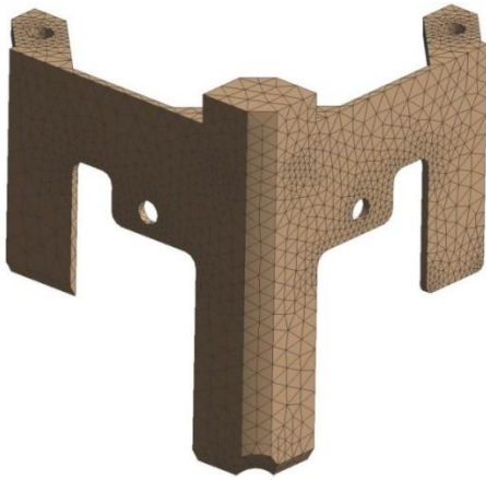
Figure 6-2 Channel fastener mesh
