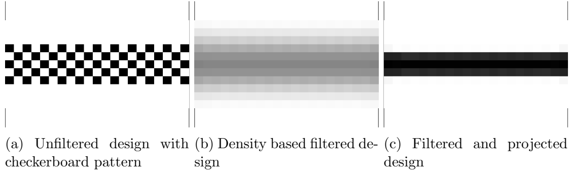
Figure 2.5: Showing the effect of the filtering technique and projection on a simple linear design
