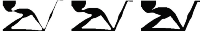
Figure 2.8: Example of a projected eroded, intermediate and dilated design in the order from left to right.
