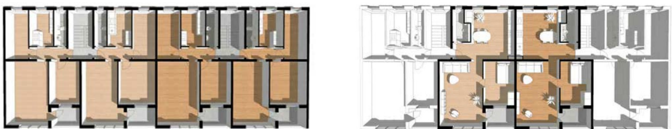
Figure 14: Original layout (left) and typical transformation (right) of a floorplan in a residential building from the 1950 [BeDa14]
