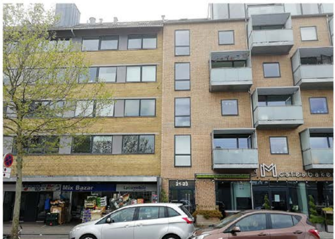
Figure 64: Reference for the combination of old and new fabric. The particular surface pattern of new bricks creates an interesting texture and a nice contrast to the existing brick wall. New windows adopt the frame colour and width of the existing windows, while the new windows extend to the floor.
