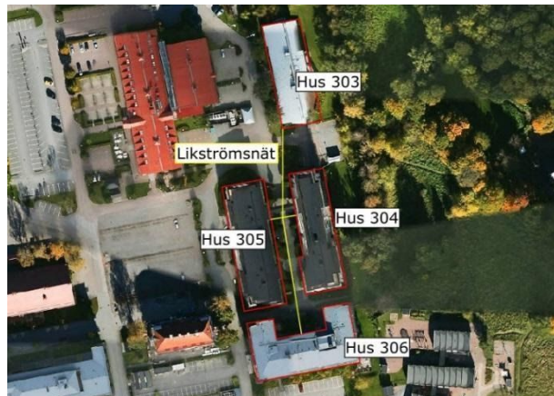
Figure 2: Aerial photo of the area in Uppsala science park with the LVDC distribution grid coloured in yellow (Flyckt, 2018).
