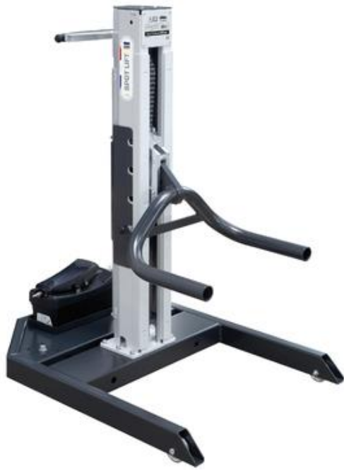
Figure 4.21 Vehicle lift, hydro-pneumatic lift, max 2500kg (GYS, 2020).
