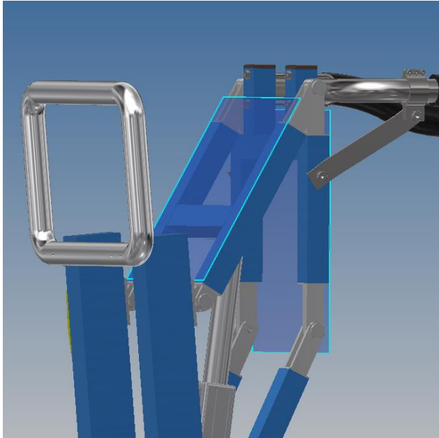
Figure 7.32 Two plastic sheets for protection (the two outlined blue transparent rectangles).
