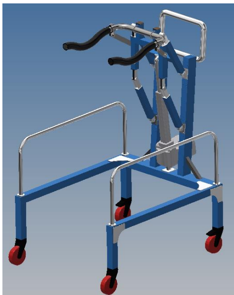
Figure 7.30 Image showing the three support tubes.
