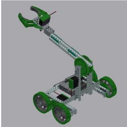
Figure 4.23 Example of rotating joint lift design (VEX Robotic Competition, 2020).
