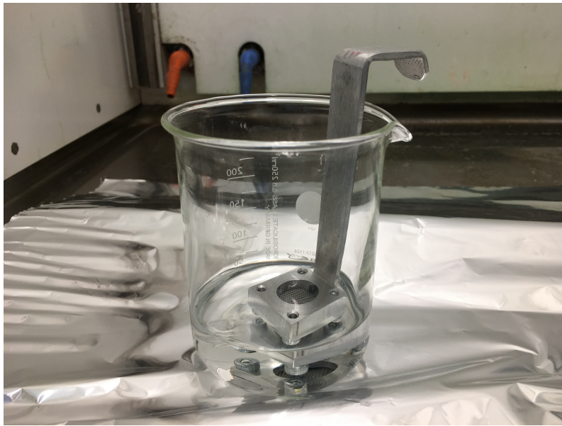
Figure 46: The sieve lowered into an acetone solution.
