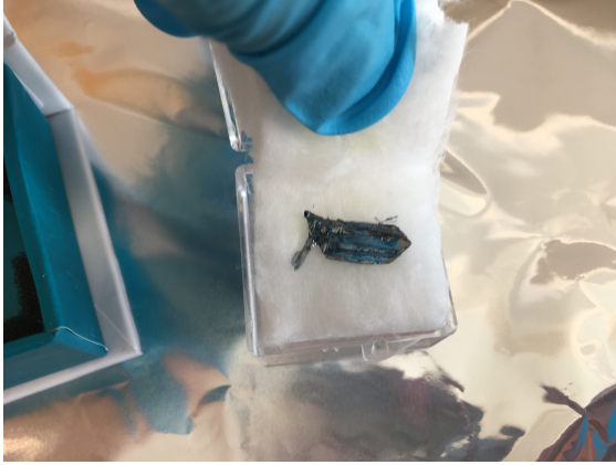
Figure 12: The bulk piece of black phosphorus used for exfoliation. When not used, is stored in vacuum in a dark container.
