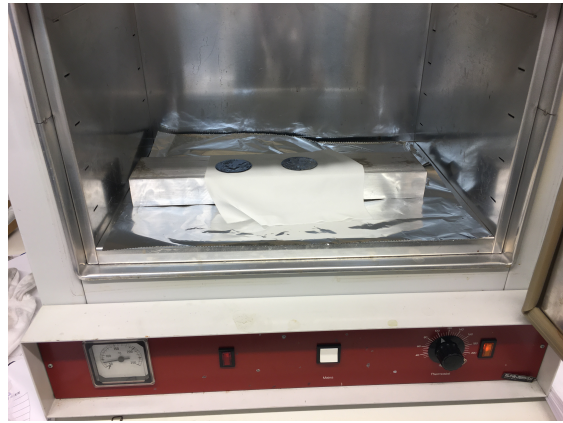
Figure 25: The PMMA film is baked for 2 hours in an oven.
