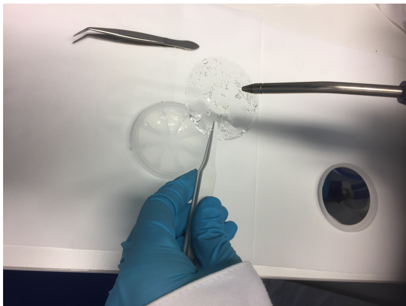
Figure 28: The wafers and PMMA films are dried gently with pressurised air.
