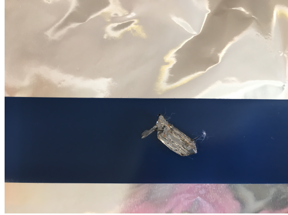
Figure 13: The bulk material as placed on the tape. It is placed and pressed down slightly, and then carefully exfoliated using tweezers.
