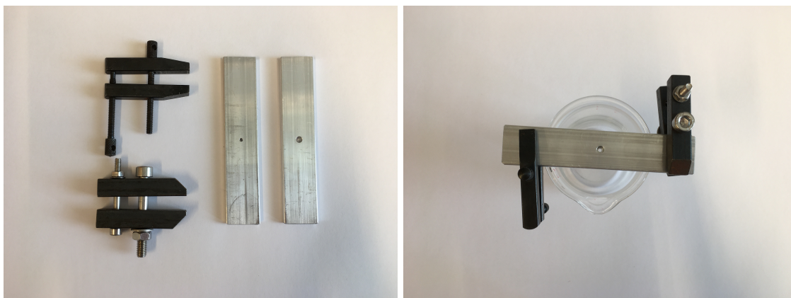
(a) The metal plates, one with a hole of 2 mm diameter and the other with 5 mm, as well as two vices. (b) The assembled product. The two vices are used to press the two metal plates together.
