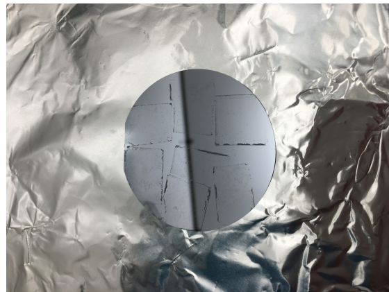
Figure 21: After cleaning, most of the tape residue has been removed, except for the thicker areas that were along the edges of the tape pieces placed on the wafer.
