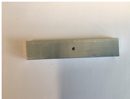
(b) The plate with the 5 mm hole is placed over the grid. The grid can be seen in the hole.
