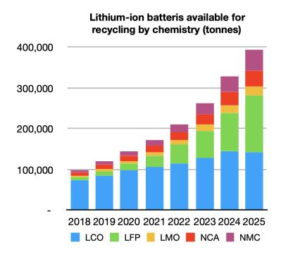
Figure 14: LCO and LFP will be the dominant cathode chemistries reaching EOL until 2026 globally [1].
