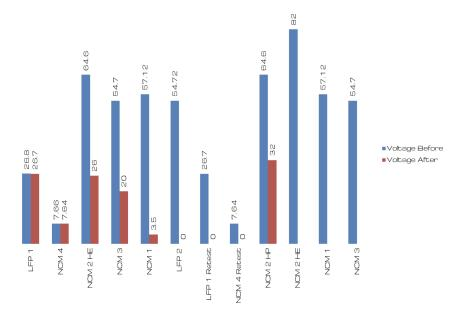
Figure 19: Cells may have residual voltage, even after fire tests, figure copied from [14]
