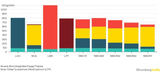
Figure 12: The mass per kWh for different type of chathode chemistries. Copied from [9].
