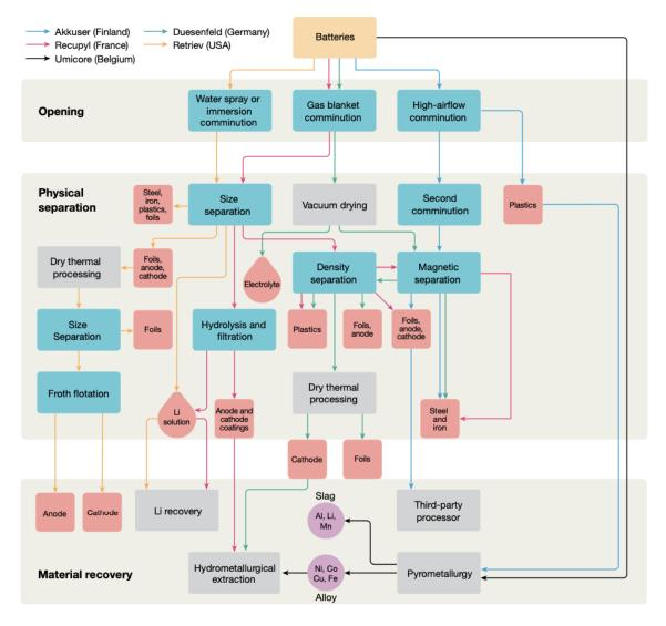
Figure 24: A flow chart of the recycling methods used by different recyclers [8]
