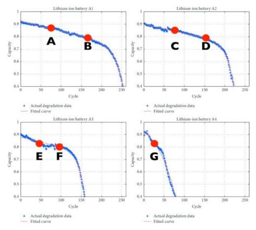
Figure 3: Degradation curve of 4 different lithium ion batteries. The value is higher the more remaining capacity. For example, Batteries at A,C and E are more valuable than at B,D,F and G. Figure adopted from [3], but modified by the author.
