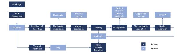
Figure 23: Pretreatment process. Modules are either thermally treated with a resulting slag going to further recycling, or crushed and separated into black mass, going to further recycling. Adopted from [17, 18, 19]. \*Binder separation has only been found in [18].
