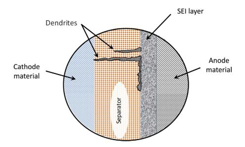
Figure 18: Dendrite formation on SEI may penetrate the separator, causing an internal short circuit. Copied from [12].
