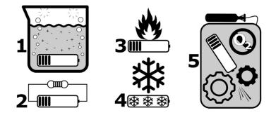
Figure 25: Five methods to stabilize a battery before comminution [20]
