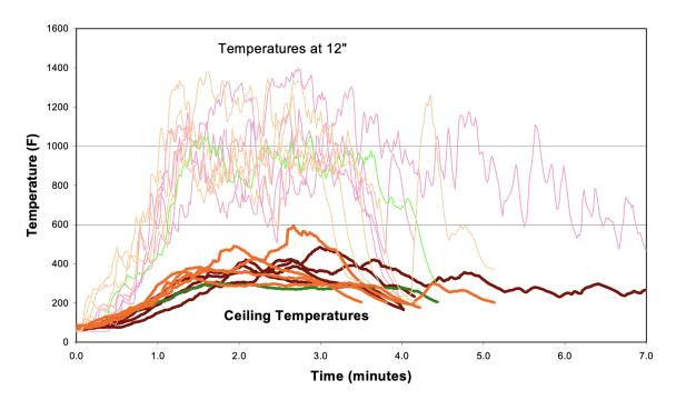
Figure 17: The peak temperature of a of LIBs venting with fire, measured in Fahrenheit and 12 inch from the chamber floor. Copied from [13].
