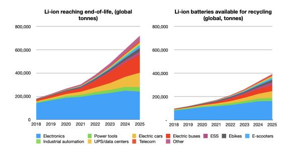
Figure 4: Roughly 50% of the lithium ion batteries that reach end of life are available for recycling. [1]
