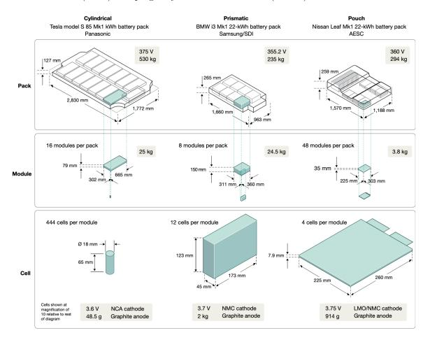
Figure 10: There many different types of EVBs and modules, but they are all based on three types of cell geometries. The dimensions and shapes varies greatly. Copied from [8].
