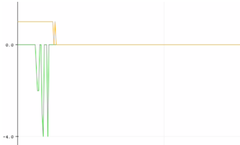
Figure 5.7: A plot showing the motion indication in binary (yellow) and the signed velocity (green) in km/h over time.
