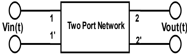
Fig. 4. Two-port network floating input and output ports.
