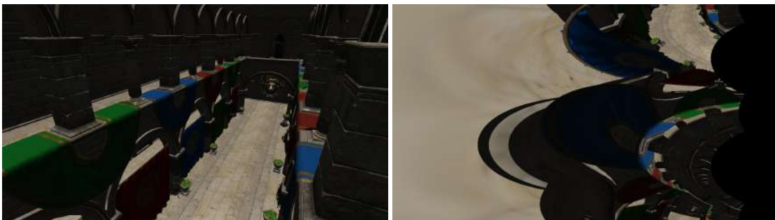
Figure 2.1: The left image is ray traced using one ray per pixel. The right image shows the same view in log-polar space.
