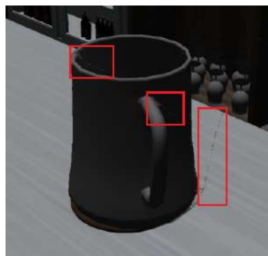
Figure 5.5: Figure illustrating the ghosting, contained in the red rectangles. The camera is moving towards the right.
