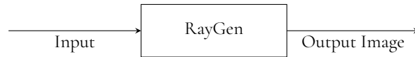
Figure 4.1: The dataflow when rendering using RayGen . The output image is either the ground truth image or the basic ray tracer’s output image, depending on which of them is in use.
