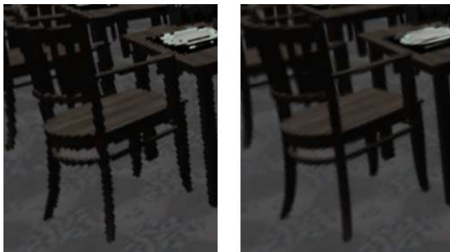
Figure 3.5: In the left image, there is no variation of the rays. The right image uses the Halton sampling pattern. Both images show the same section of the periphery from one specific view.
