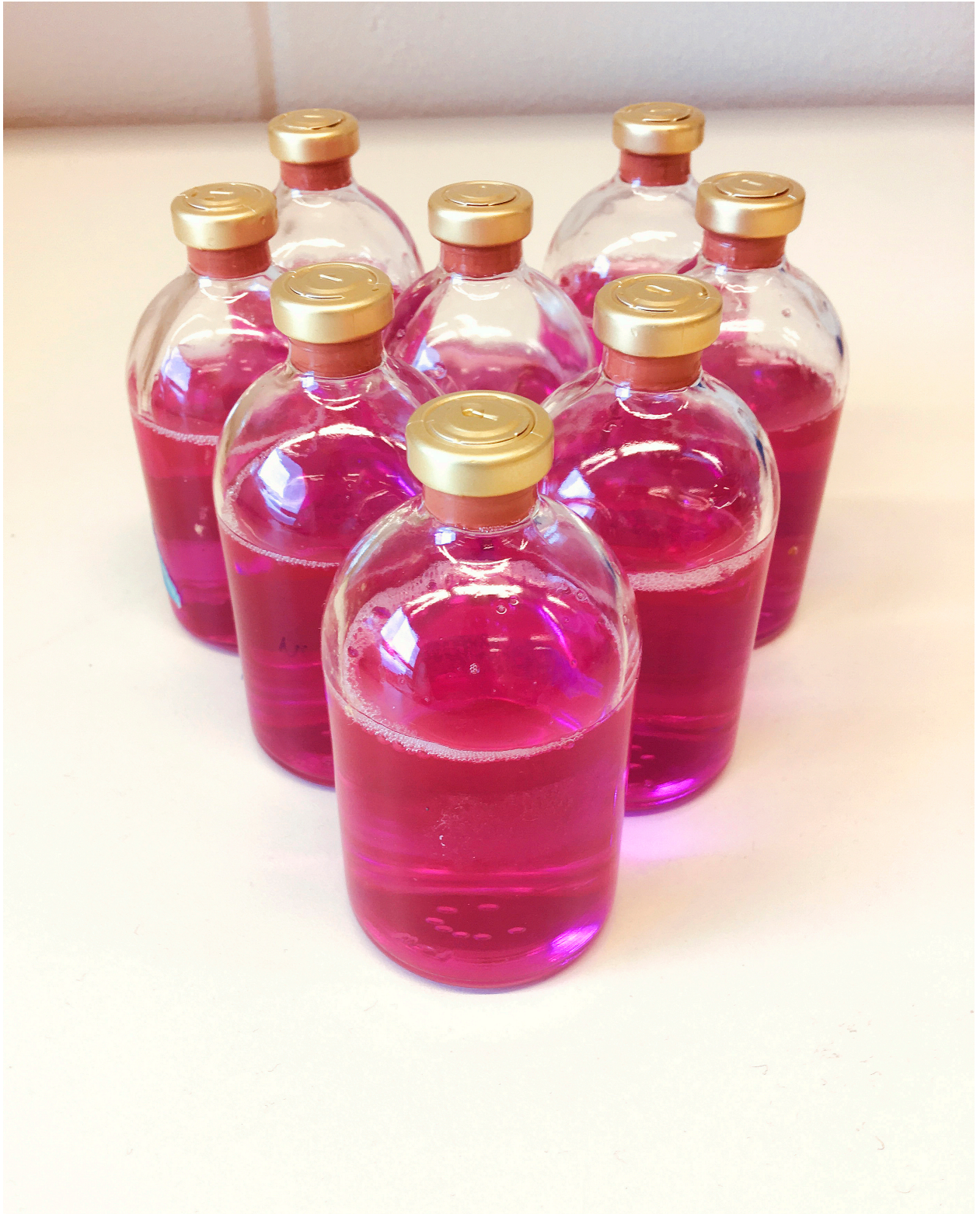
Figure 7. DMMG prior to autoclaving. The intense pink colour is due to the redox indicator resazurin, which becomes colourless after the heat treatment.
