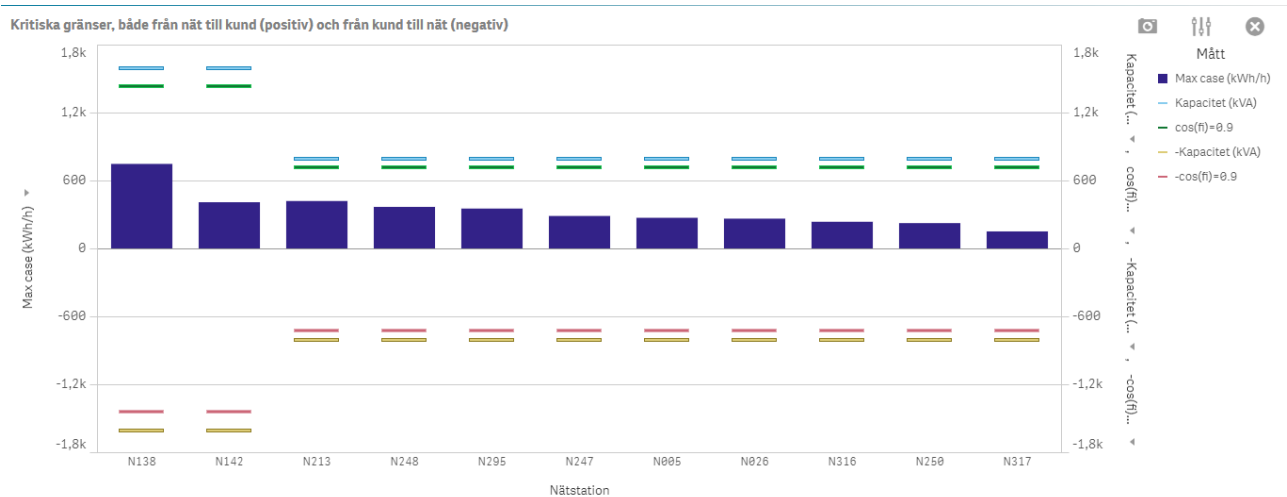
(a) Maximum load per secondary substation with a solar power installation with 500 kW peak power
