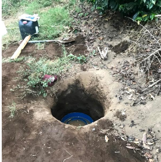
Figure 8. Setup of a double-ring infiltrometer below ground surface.
