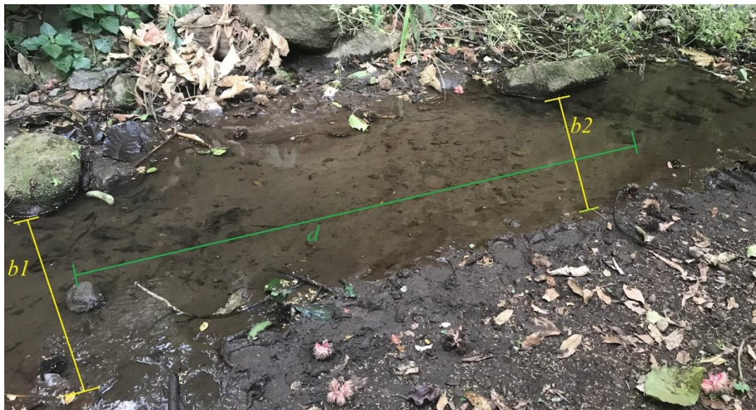
Figure 9. The parameters b_1 , b_2 , and d shown visually, note that the endpoints of the section d do not necessarily have to coincide where the stream width is measured.
