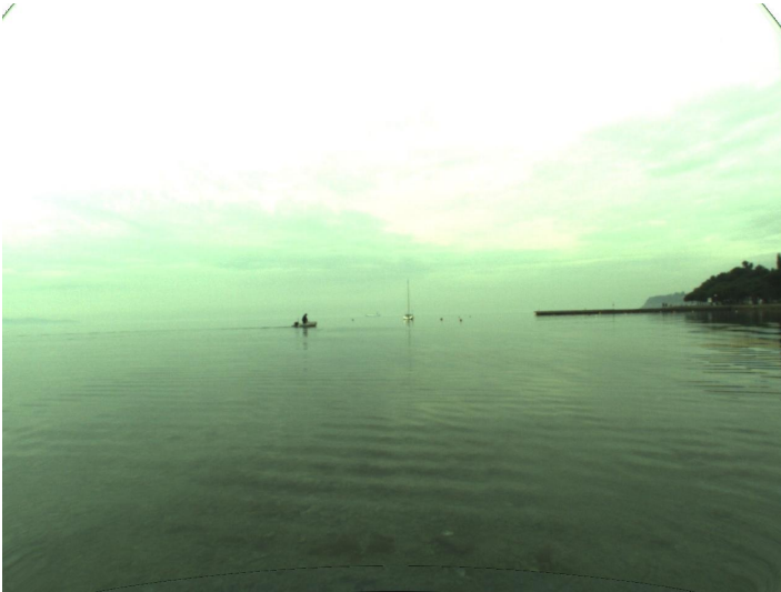
Figure 7.3: An image from the MODD2 dataset demonstrating the issue with using it as a performance indicator for obstacle detection. The image contains three evaluated objects, of which all are buoys, i.e., the two boats are not counted.
