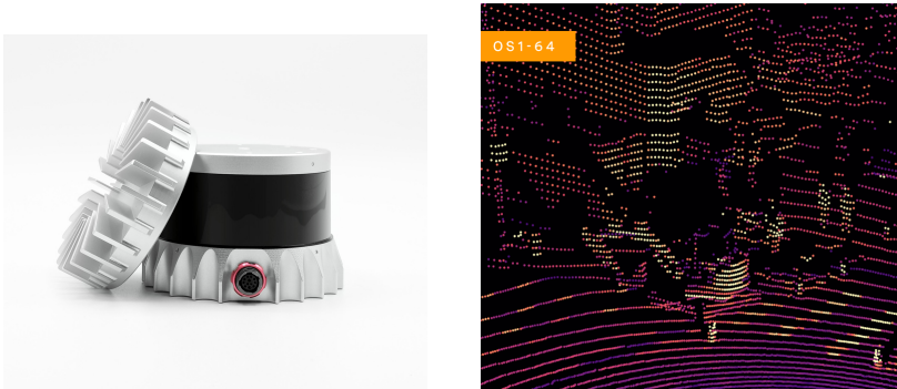
(a) An example of a 3D LiDAR, Ouster OS1. (b) Visualization of the pointcloud generated from a 3D LiDAR.
