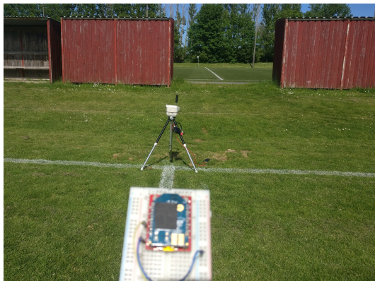
Figure 3.24: Test setup with a directional antenna and an Xbee device.
