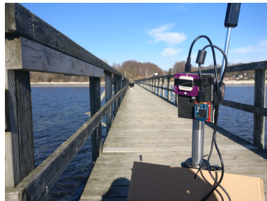
(b) Setup of one of the u-Blox NEO-M8N GNSS receivers during the test.
