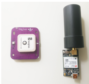
Figure 3.6: The two GNSS modules. NEO-M8N on the left and ZED-F9P with its Helix antenna on the right.
