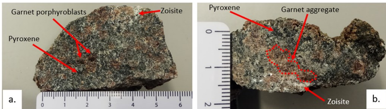
Figure 28. Hand sample of garnet-rich mafic knob in a marble-amphibolite contact zone (sample CM19R-11k). a), b): Rough surfaces of two separate pieces of the rock with distinguishable minerals of the main assemblage. The garnet rims are very thin thus, not visible even using the hand lens; however, the porphyroblasts are visible, and sometimes the clinopyroxene inclusions through very close observation.
