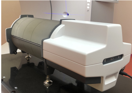
Figure 7: Representation of Delta 4 + phantom (ScandiDos, Uppsala, Sweden) positioned on the couch for plan delivery
