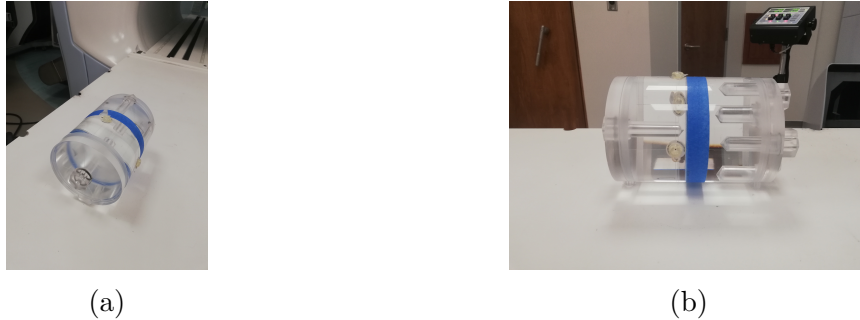
Figure 11: The ViewRay Daily QA phantom used for the daily image acquisition dataset.
