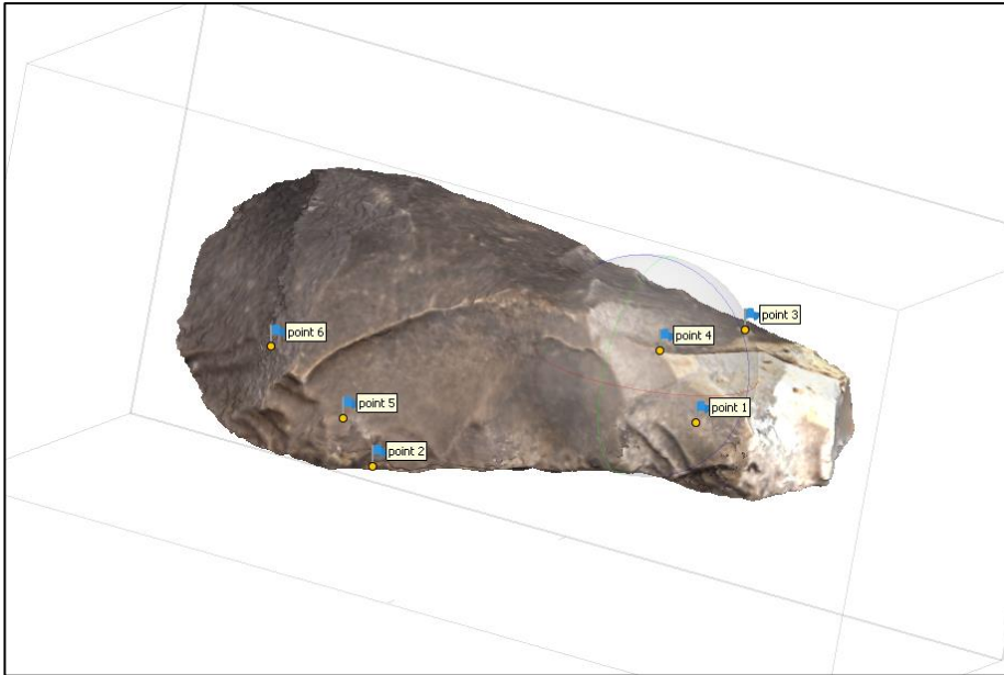
FIGURE 10: FINAL TEXTURED MESH OF FIRST SAMPLE ARTEFACT, THE CORE-AXE, SHOWING THE LOCATION OF THE ALIGNMENT MARKERS
