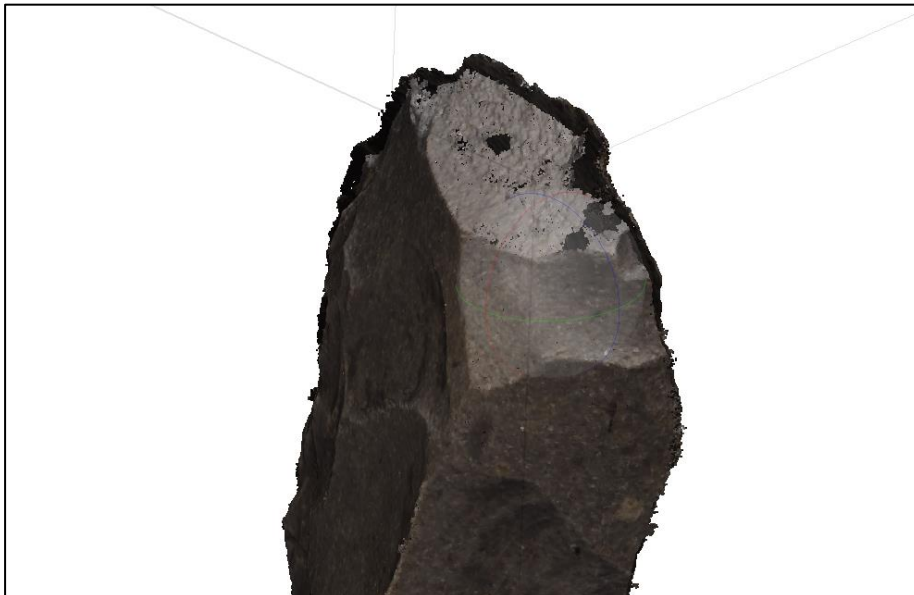
FIGURE 9: WARPED, OVERLAPPING EDGES RESULTING FROM MISSING DATA
