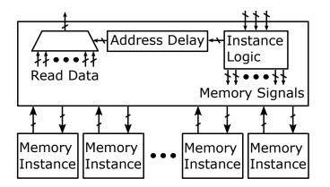
Figure 4.2: Memory wrapper structure with memory instances connected to the control logic
