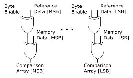
Figure 4.3: Generation of comparison data with two layers of XOR gates when byte enable is active low.
