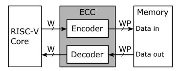
Figure 2.5: ECC parity code embedded with data
