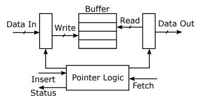
Figure 4.4: Circular buffer with read and write pointers
