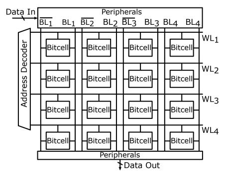
Figure 2.3: SRAM memory array connected with address decoder and other peripherals
