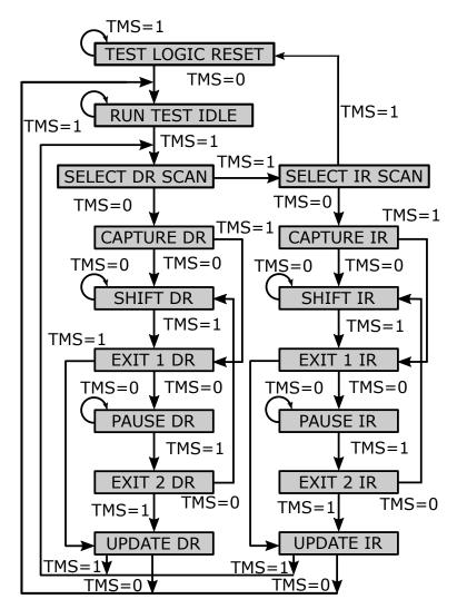
Figure 2.9: JTAG tap state machine used to control JTAG operations
