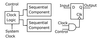
Figure 2.8: System level and fine grain level clock gating
