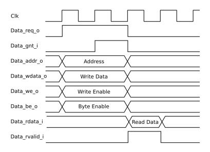
Figure 4.11: Cv32e40p RISC-V memory interface operation
