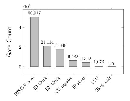
Figure 5.10: Gate count for the important blocks within the SoC system.
