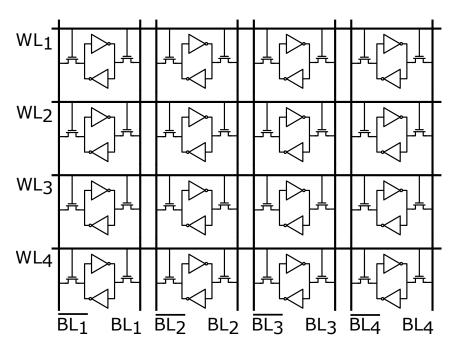
Figure 2.2: 4x4 SRAM bitcells connected to build a larger memory bank
