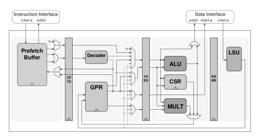
Figure 4.10: Cv32e40p RISC-V core image from [1]
