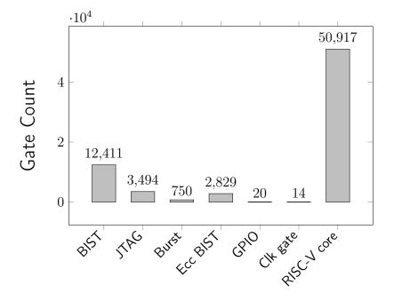
Figure 5.8: Top level gate count for the the complete SoC system.
