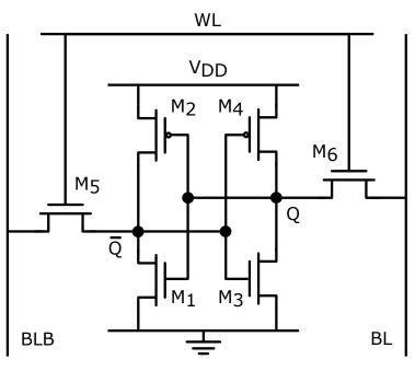
Figure 2.1: Standard 6-T SRAM bitcell
