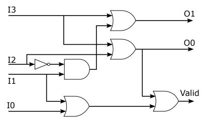
Figure 4.5: 4 input priority encoder circuit
