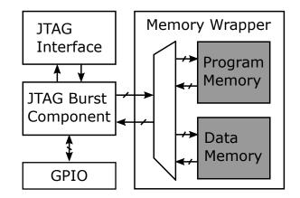
Figure 3.1: JTAG burst component integration with memory and JTAG controller.
