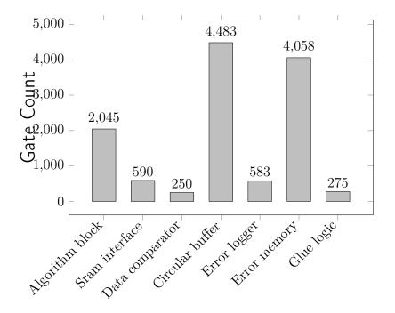
Figure 5.9: Gate count for the important blocks within the BIST system.
