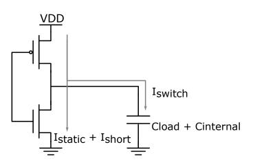
Figure 2.7: Standard inverter to demonstrate different power consumption components of circuits.
