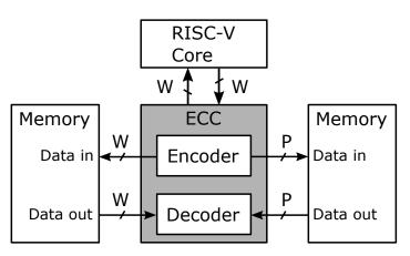
Figure 2.6: Seperate memory used to store ECC parity bits
