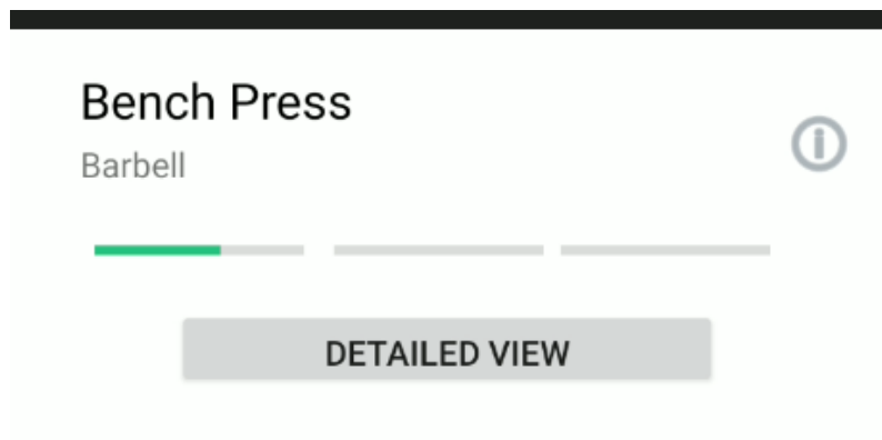
Figure 8.1. The grey colour of the button has shown to be a poor design choice with low clickability.
