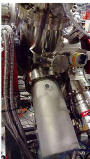
Figure 5.2: The backside of the Scienta-spectrometer chamber, where the cluster beam was caught with a mounted cool trap filled with liquid nitrogen.
