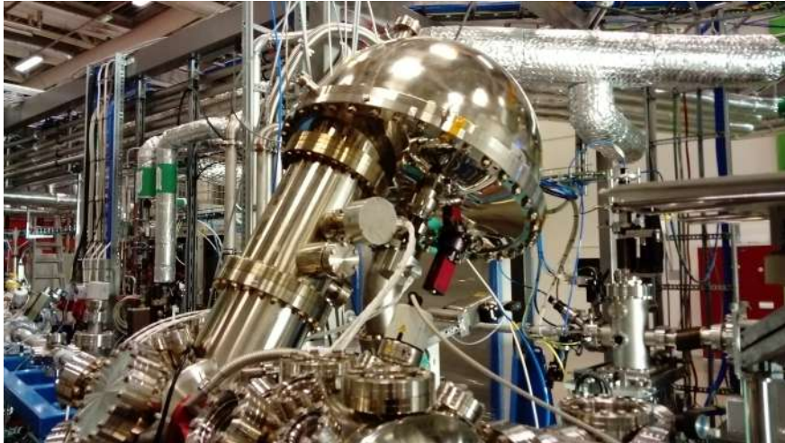
Figure 4.9: The Scienta 4000 energy analyzer as seen externally
