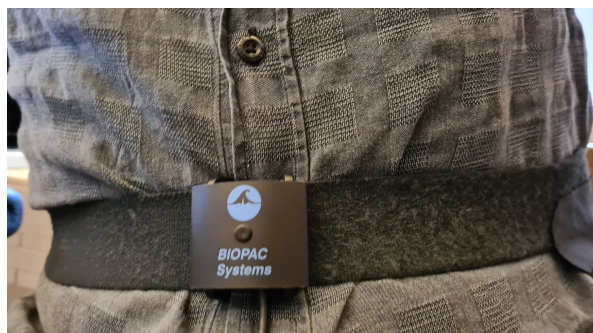
Figure 4. Respiration belt transducer attached around the abdomen.
