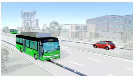
Figure 1: Electric rail placed on a road, charging a bus.
