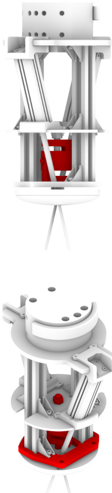
Fig. 53-54 Planned load cell integration
