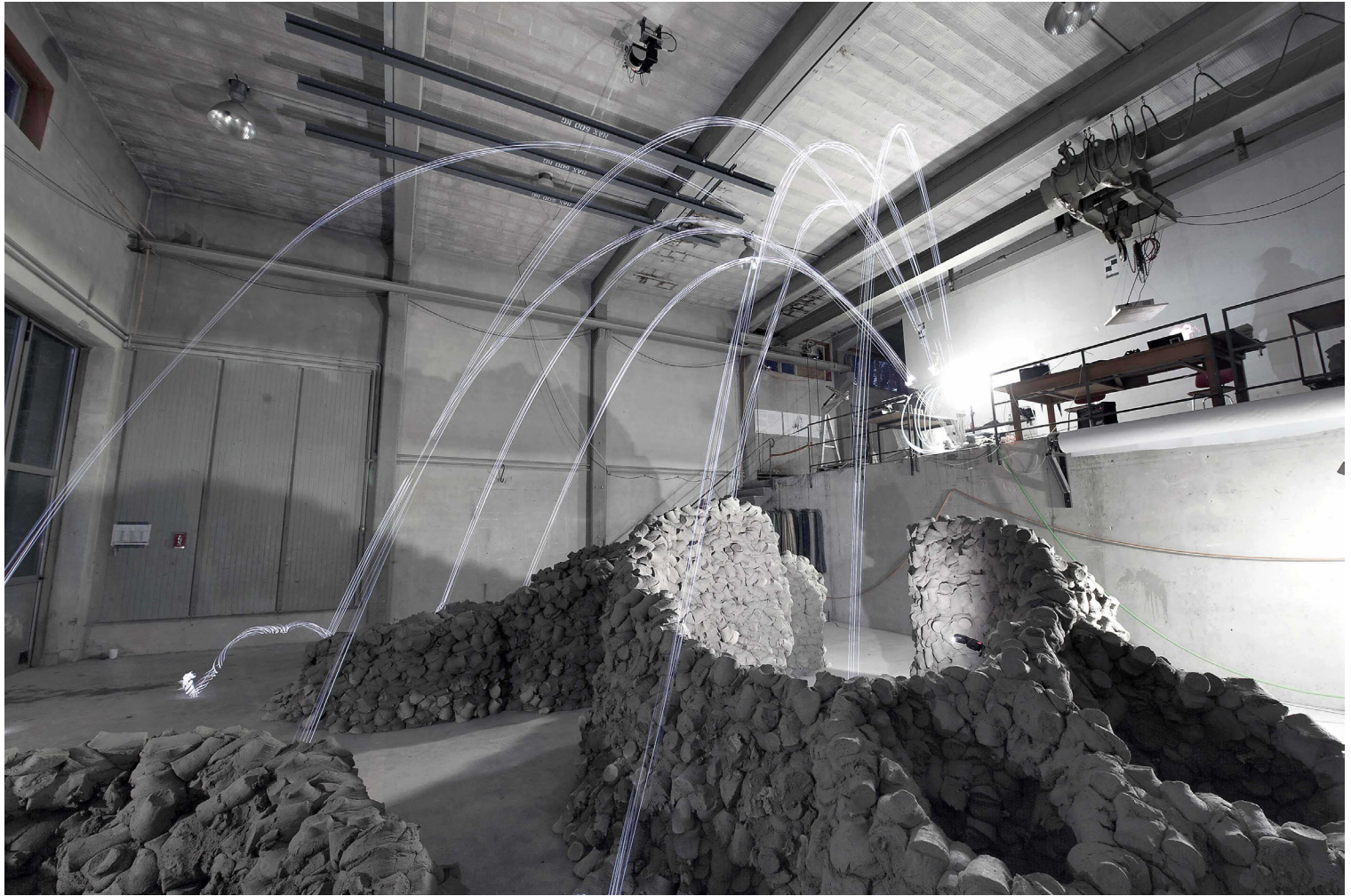
Fig. 5 Ballistic trajectories of light projectiles through bulb exposure, Remote Material Deposition Gramazio Kohler Research, ETH Zurich, 2014 © Gramazio Kohler Research, ETH Zurich
