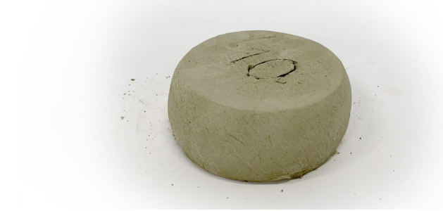
Fig. 22-23 Landquart and Berg clay tests (respectively)—example of fragmentation and plastic behavior
