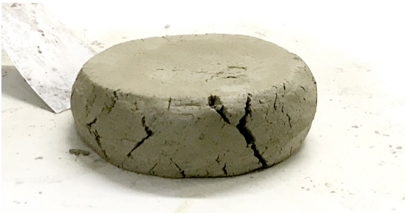
Fig. 22-23 Landquart and Berg clay tests (respectively)—example of fragmentation and plastic behavior
