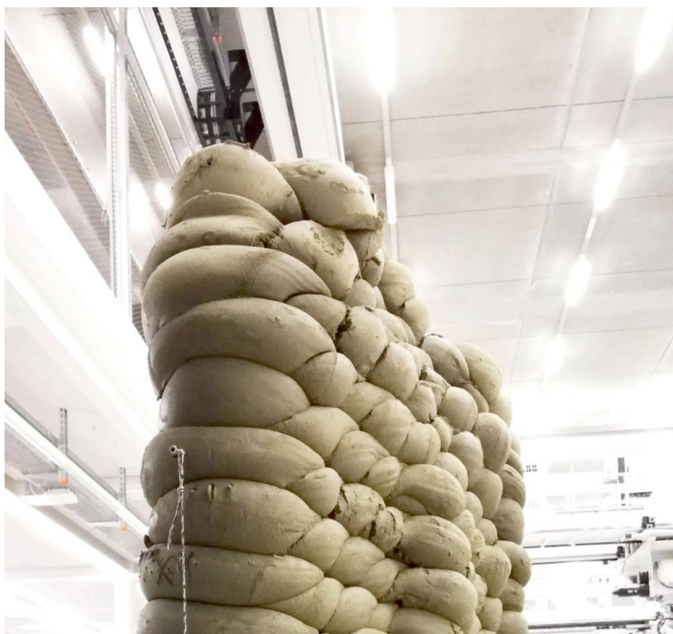
Fig. 44 Example of deformation due to shrinkage from MAS DFAB 19/20 RCF.
