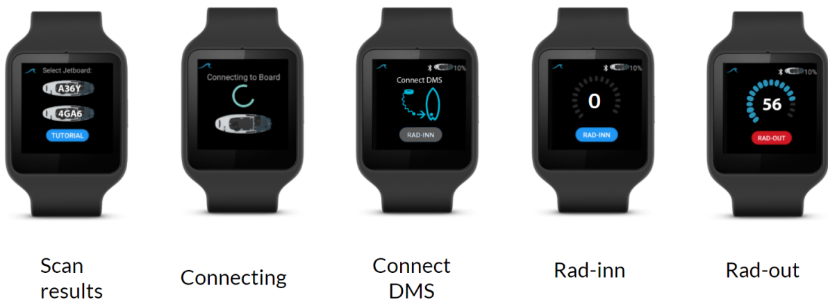
Figure 9.2: The image illustrates the flow of the UI from left to right. The surfer begins the session by touching a jetboard icon, presented in the nearby Scan Results, to connect. Whenever the surfer falls and the Bluetooth connection is lost, it will reconnect as the surfer swims closer to the jetboard. Connect Dead Man's Switch (DMS) view notifies the surfer if the dead man's switch requires attaching to the jetboard. Once safety is assured, the smartwatch application recognises hand gestures to activate (Rad-inn) and deactivate (Rad-out) the speed manipulation and to manipulate the speed. The UI displays jetboards in the vicinity, connection, battery, engine activation, speed, and dead man's switch statuses.
