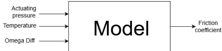
Figure 11: BorgWarner MISO friction model.
