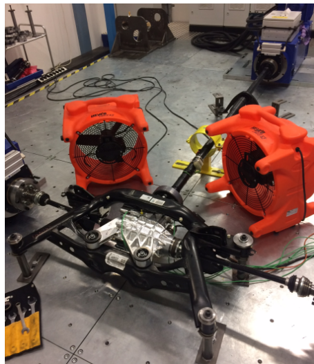
Figure 13: A full clutch and differential test setup.
