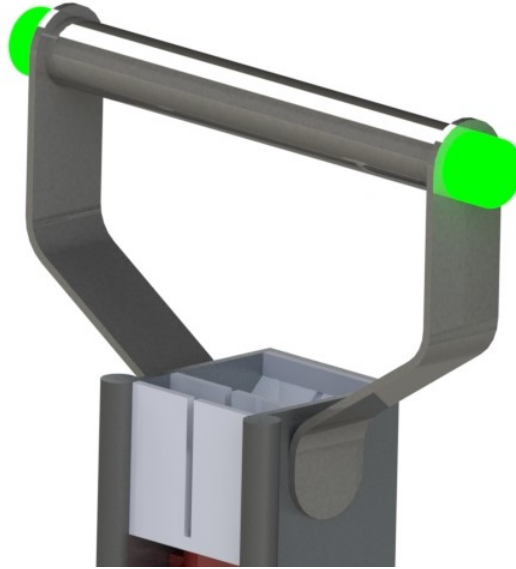
Figure 6.14: Handle with feedback lamp on top of receiving stand.
